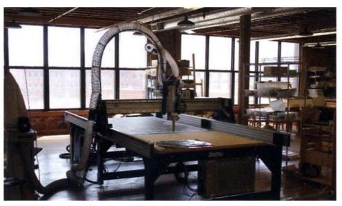
Figure 177. Large ShopBot router at Mike Lyon's studio in Kansas City. The router is set up to hold an ink pen that is raised and lowered via a custom solenoid headstock designed by Lyon. Image courtesy of the artist.
